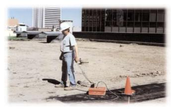
The instrument consists of a transportable field electromagnetic impulse transmitter and receiver, which emits impulses that are reflected back to the receiver. The returned impulse-variations are presented as hyperbolic patterns, caused by the reflection changes, and are displayed graphically on a strip chart. This provides paper documentation and gives a continuous record of the subsurface under the track of the antenna.
